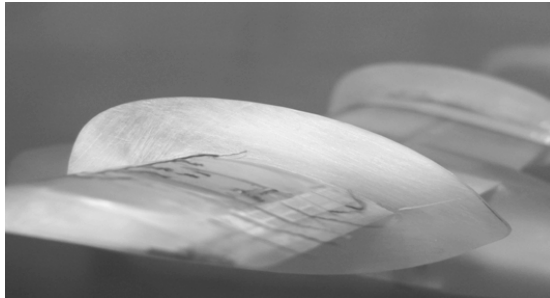
Fig. 12 a) Time trace of the shear stress sensor output; b) tufts flow visualization over the wingtip. \alpha = 8.5 deg, synthetic jets off.
